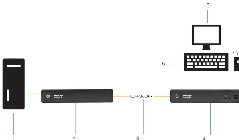
FIGURE 2-1. EMERALD EXAMPLE – UNMANAGED BASIC INSTALLATION
